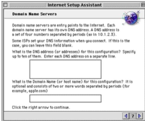
**On the first line of the large box, type 63.90.84.3 and return. (default DNS IP address)**
